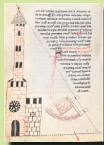
Fig. 13. A plumb dangling from a line yields the angle.
